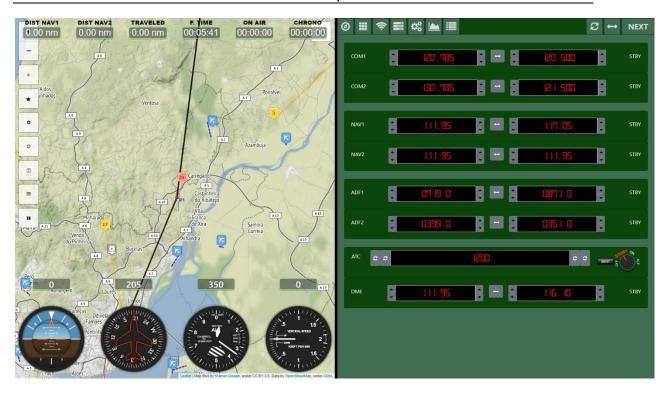
The radio panel consist of seven individual radio devices plus the transponder device.
