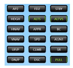
The autopilot widget in the PFD contains all the autopilot buttons to interact with. It has two modes: push and pull. Basically, two available sets of buttons switched from the last bottom right button in the grid.
